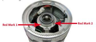
Therefore turn the grind adjustment of the built-in grinder to the right red mark 2 for refitting the grinder's lid.
