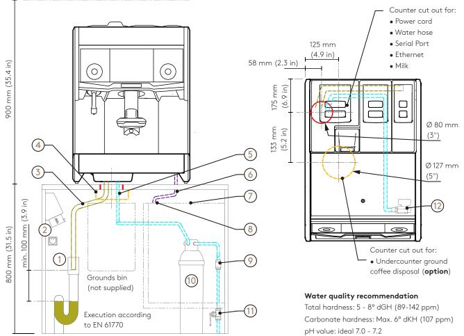
Min. height required to refill/remove bean hopper
