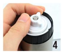
Adjust the grind by turning the adjustment nut clockwise for finer and anti-clockwise for coarser.
