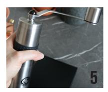
Secure handle to the top nut and begin grinding, making sure to keep the handle level.
