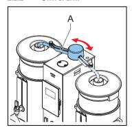
The swivel arm (A) directs hot water from the coffee brew system into the top of a distributor lid.
