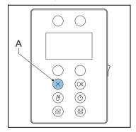
The stop button (A) stops the brewing process. The machine is still charged after the brewing process is stopped. Unplug the machine to make sure that the machine is entirely uncharged.
