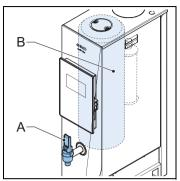
CB models with a 'W' designation in the model name, have a hot water tap (A) to serve hot water from an additional boiler (B) inside the tower.
