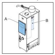
The user selects a desired quantity of beverage on the control panel (A). The coffee brew system (B) inside the tower heats the corresponding quantity of water.
