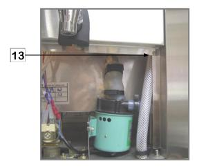
panel away from the plastics. Lift the Front Panel away. All the internal components are now accessible.
