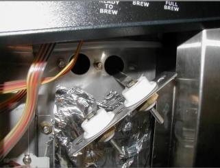
Removal of the Low and High Level Probe assembly
