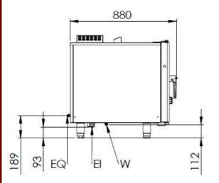
EI=ELECTRIC INLET EQ=GROUNDING CONNECTION W= WATER INLET
