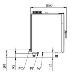
EI=ELECTRIC INLET EQ=GROUNDING CONNECTION W= WATER INLET
